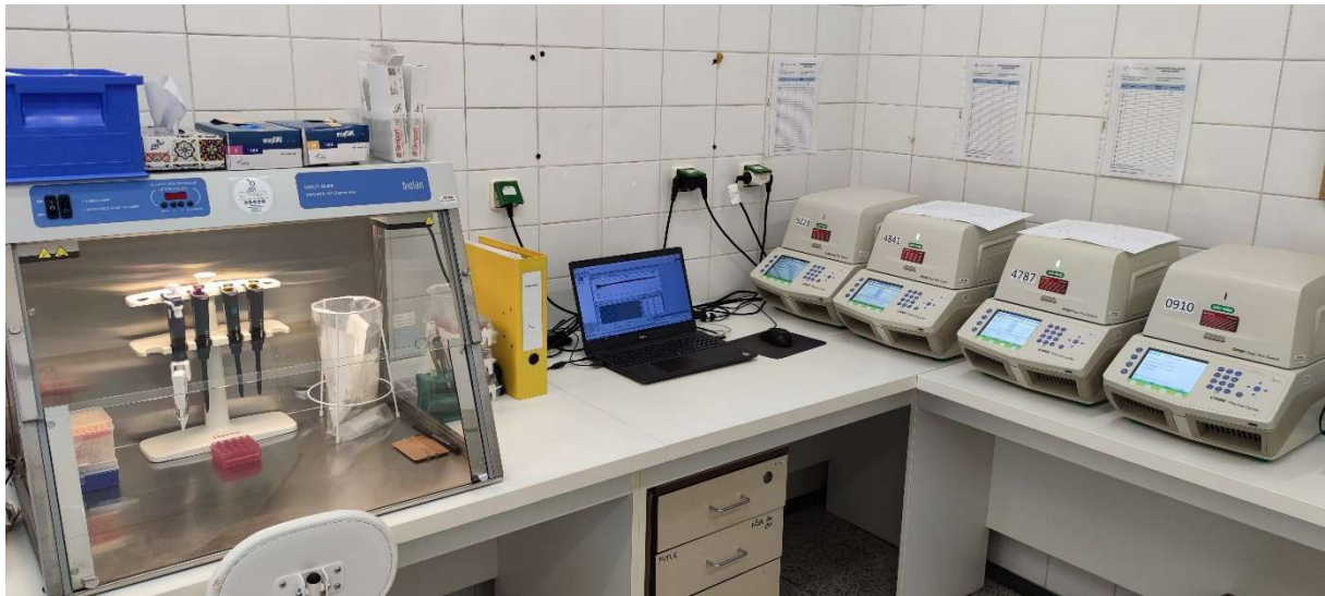
Laboratoř PCR diagnostiky – Real-time PCR thermocyclery.
